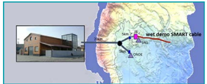
BATHYMETRY MAP OFFSHORE CATANIA SHOWING THE PLANNED ROUTE OF THE WET DEMONSTRATOR SYSTEM (HOWE ET AL., 2022)
