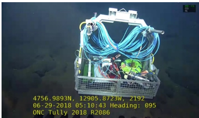
Figure 3. ROPOS toolbox containing Maris OBS, interface unit and cabling (Image courtesy of Ocean Networks Canada)
