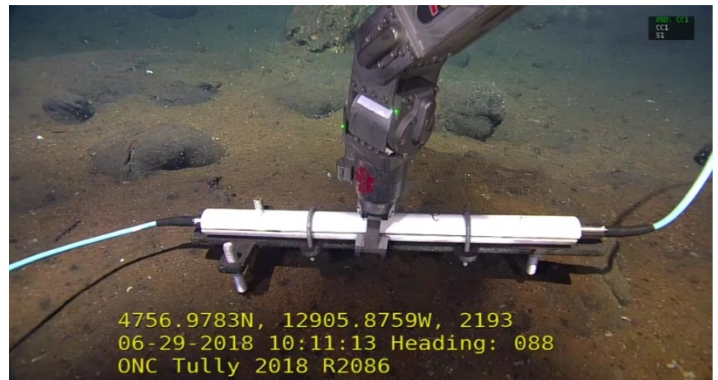
Figure 4. Güralp Maris Seismometer being placed in position at 2200m depth (Image courtesy of Ocean Networks Canada)
