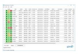
Launch Discovery software. The serial number (as shown on the base of the Minimus) should appear in the main window. If the instrument does not appear, check your Ethernet connection and then press the Scan locally button (more troubleshooting details in user's manual in section 4.1) Select the instrument and click on the View toolbar to select Live View then GDI only.
