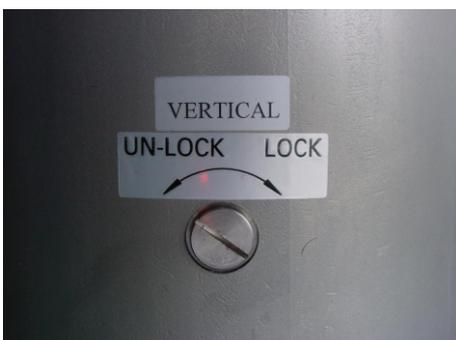
Remove the screw cap protecting the vertical lock access socket, and insert a hexagonal wrench.. Find the retaining screw within, and loosen it to unlock the vertical component. Repeat for the north/south and east/west components.
