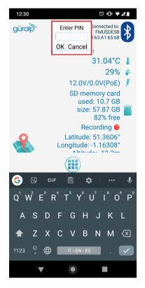
The default PIN code used to access the Instrument Control menu is "0000".
