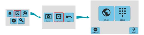
The network page allows you to choose between DHCP mode, where the networking parameters are set by an external DHCP server, or static mode, where the network parameters must be typed in manually.
