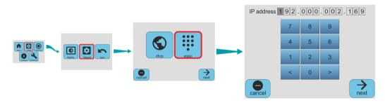
Enter the desired IP address using the on-screen virtual numeric keypad and then press "next", which takes you to the netmask screen.
