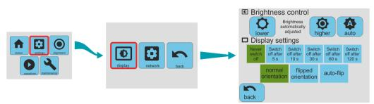
The "display" page allow control of brightness, the inactivity time-out and the orientation of the display.
