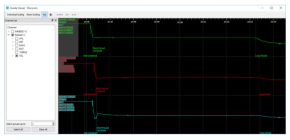
When the auto-centring is enabled, the centring procedure is activated as soon as the percentage reaches ±100%. To turn off Automatic Mass Centring, select the
