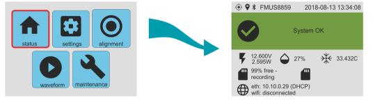
The "status" page shows information about serial number, Bluetooth status, time and date, GNSS/PTP status, input voltage and power, humidity, temperature, microSD cards recording status, I.P. address.
