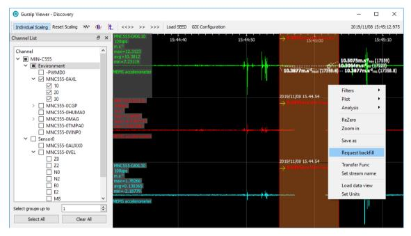
The gaps are backfilled automatically for all the streams selected, if the requested data is available in the microSD card.
