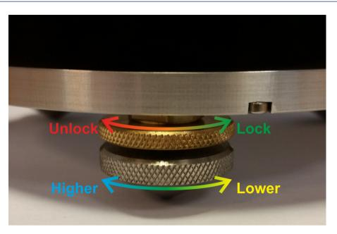
The feet are mounted on screw threads. To adjust the height of a foot, turn the brass locking nut clockwise (when viewed from above) to loosen it and rotate the entire foot so that it screws either in or out. When you are happy with the height, tighten the brass locking nut anti-clockwise to secure the foot.
